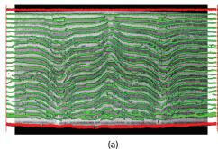
Figure 26. Ultrasonic analytic signal imaging for a specimen containing numerous aligned tape gaps and overlaps, causing outof-plane wrinkling: the X-ray CT image (a) has an overlay inverted from the analytic signal response (b), where red lines are the front and back surfaces, while the green lines are the resin layers between plies, all determined automatically from the ultrasonic full-waveform data<sup>[2]</sup>
