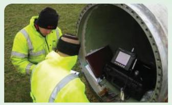
Figure 21. Field inspection using eddy currents of the blade can bolt holes
