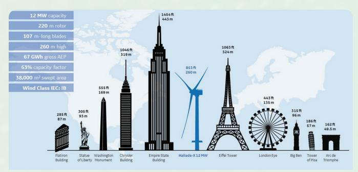
Figure 1. Comparison of the GE Haliade-X 12 MW wind turbine with other well-known structures
