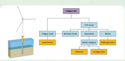
Figure 10. Various parameters affect the fatigue life of the asset
