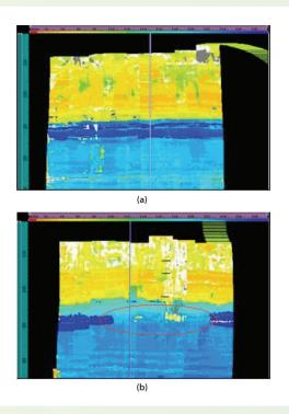
Figure 19. C-scan of internal web-to-blade-skin bonding: (a) wellbonded web (dark blue strip); and (b) disbonded web (circled)
