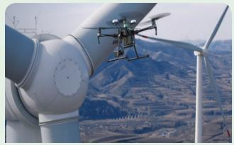
Figure 17. Drone visual inspection
