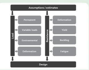
Figure 9. In the early stages of design, assumptions and estimations are made as to the loads experienced by the structure
