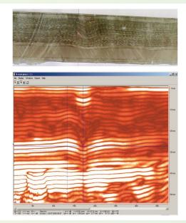
Figure 23. Example of a wrinkle in a blade structure and an ultrasonic B-scan cross-section
